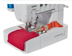
The Dual Function Fold Binder is used to fold 1.25 inch (32mm) wide bias fabric tape into 0.31 inch (8mm) wide double fold bias tape, and then apply the bias tape binding to the edge of fabric. Attach the binder to the cover stitch machine simply with the two included screws. This accessory may also be used as a binder for single fold bias tape.
